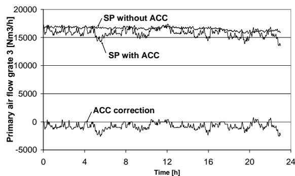
Fig. 5 Set point for the primary air grate 3.
