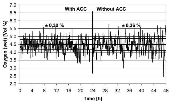
Fig. 3 Oxygen<sub>(wet)</sub> content with and without the ACC system.
