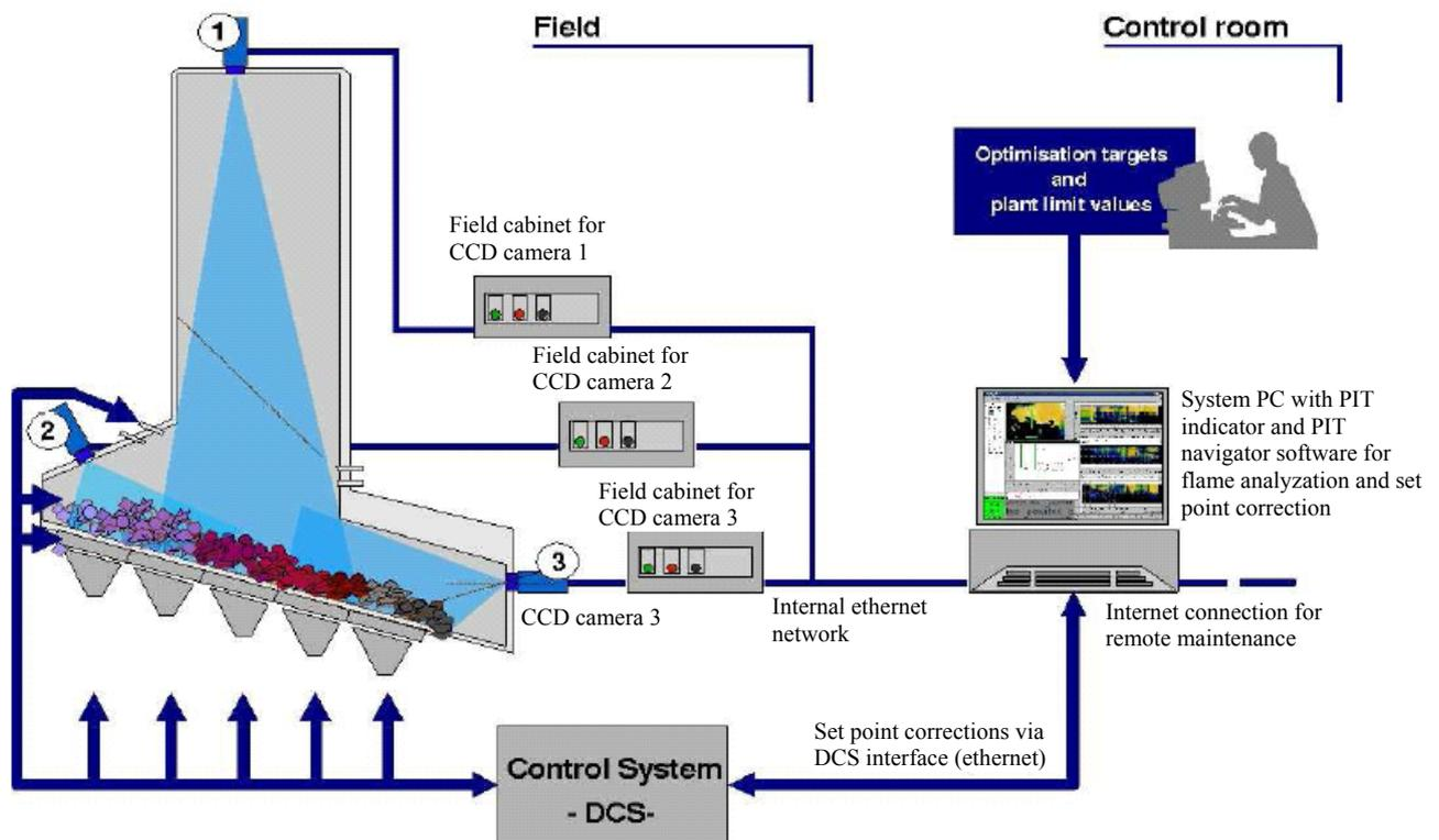
Fig. 1 Position of CCD camera at the L90 plant.
