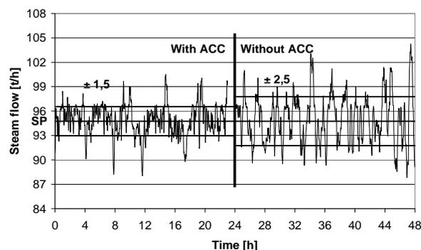
Fig. 2 Steam flow with and without the ACC system active.
