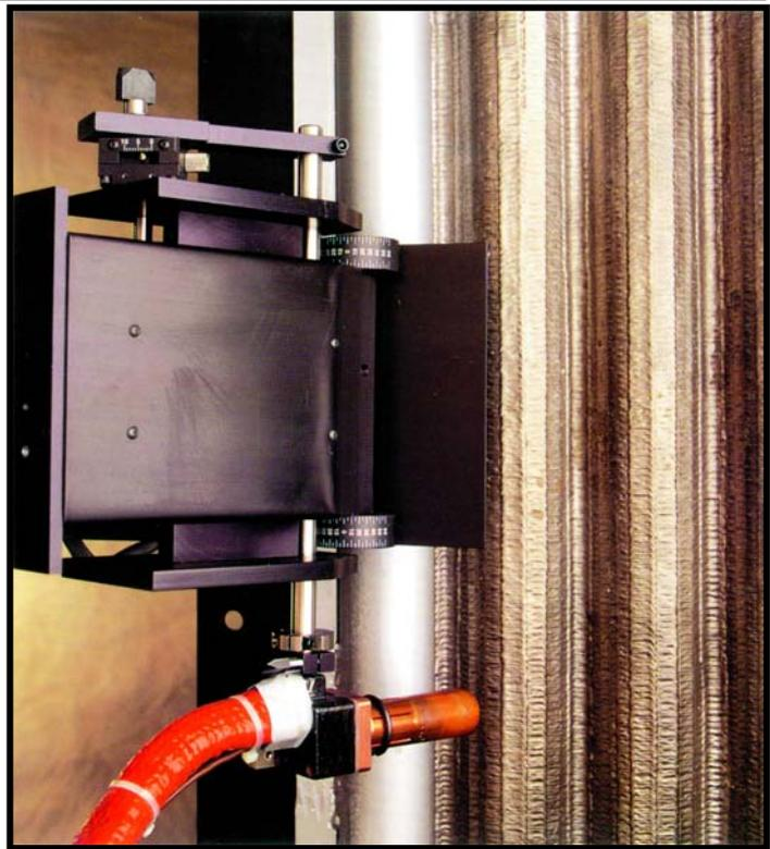
In some cases, it is recommended to carry out the Inconel cladding on site. Babcock & Wilcox Vølund has extensive expertise in this area and performs on-site semi-automatic or manual application.
