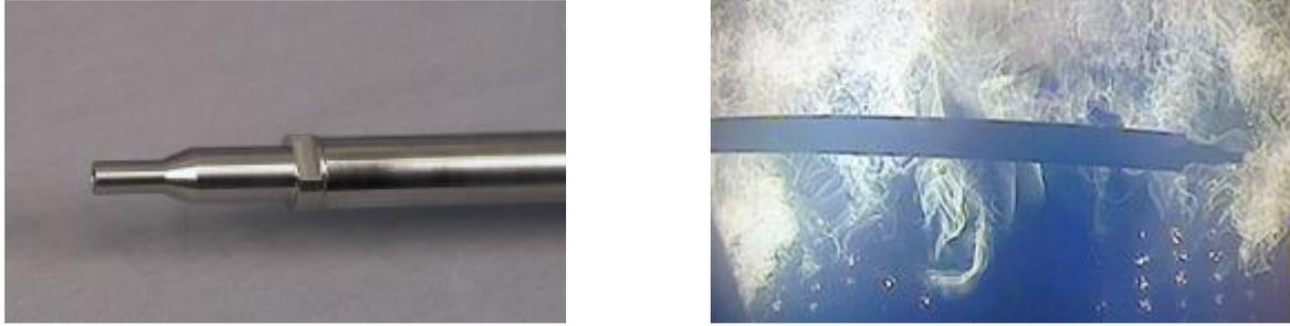
Figure 4. Left figure (a) shows the nozzle of the suction pyrometer. Right figure (b) shows the suction pyrometer inside the furnace close to the grate.
